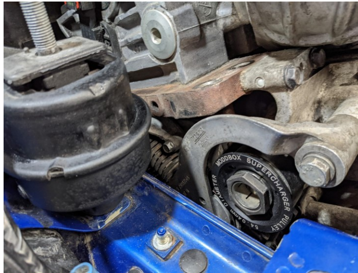
Figure 5 – Pulley, bottom-half of engine mount, tensioner, and belt installed
