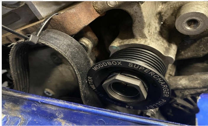
Figure 3 – Installed Moddbox Supercharger Pulley with correct offset
