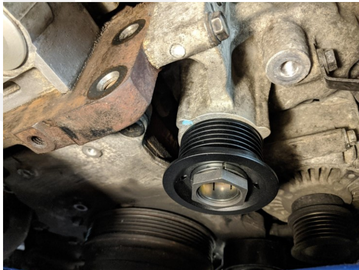
Figure 1 – Moddbox Supercharger Pulley and Moddbox Patented Pulley Drive Coupler on shaft
